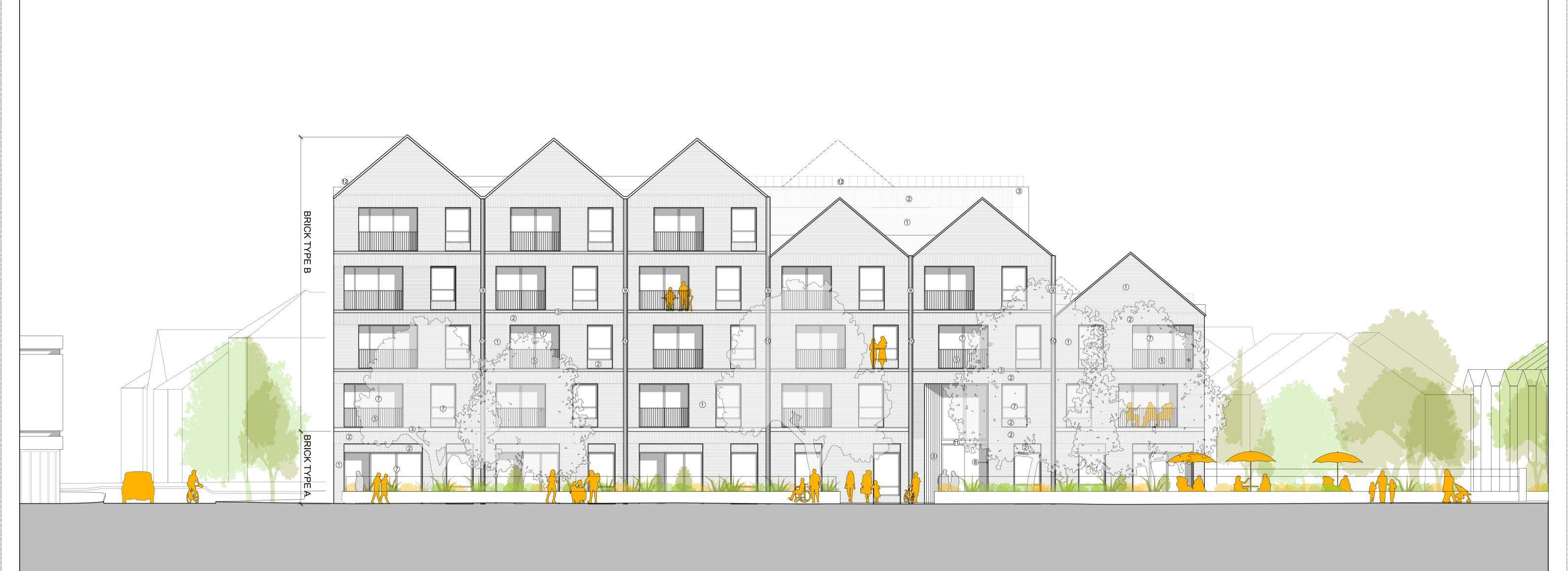
① STRETCHER BOND BRICKWORK WITH FLUSH, COLOUR MATCHED MORTAR (2 VARIETIES OF BRICK - A/B) ② VERTICAL STACK BOND BRICK WITH FLUSH, COLOUR MATCHED MORTAR (2 VARIETIES OF BRICK - A/B) PRE-CAST RECONSTITUTED STONE HORIZONTAL STRINGER/COPING - MID-TONE COLOUR AS BRICK TYPE B
